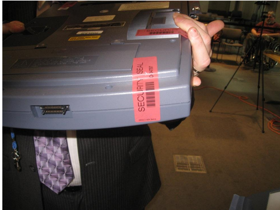
Photograph 1.4 seals on TSx case
